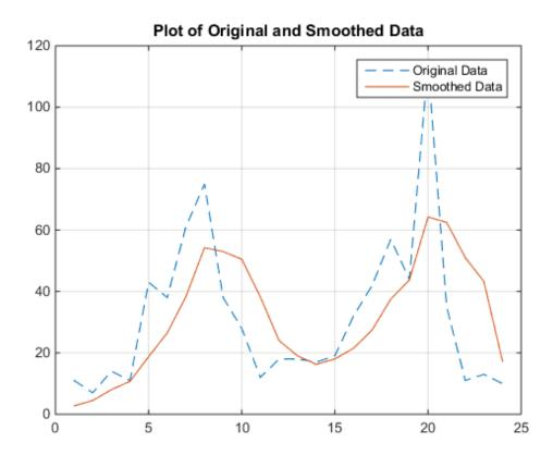
The filtered data, represented by the solid line in the plot, is the 4-hour moving average of the count data. The original data is represented by the dashed line.
