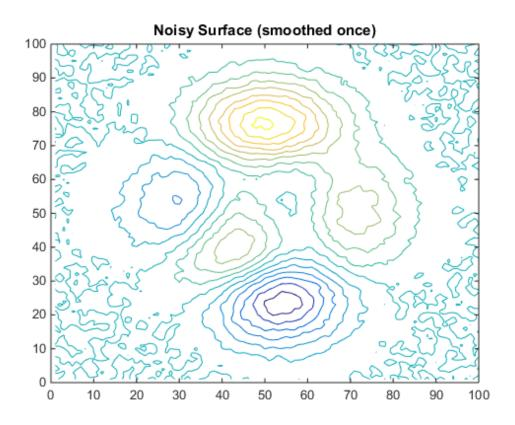
Smooth the surface one more time using the same operator and plot the contour lines. A larger or more uniform kernal can achieve a smoother surface in one pass.
