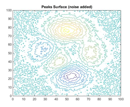
Specify a 3-by-3 convolution kernal, F, for smoothing the matrix and use the conv2 function to attenuate high spatial frequencies in the surface data. Plot the contour lines.
